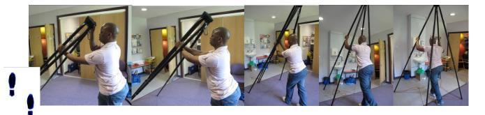
Make final adjustments – adjust height settings of legs and straighten red connecting cables
