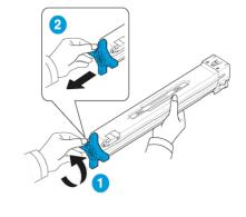
Rotate the end cap anticlockwise until it releases
