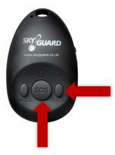
A voice memo can be left by pressing the **Call 1 button** for **three seconds.** The GPS light will start to flash to confirm the request. Speaking clearly, leave your voice message when prompted. To end the memo, press the **SOS button**.
