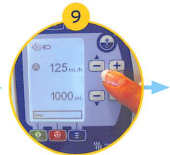
9 Set the desired flow rate by pressing the +/- keys until the desired volume is reached
