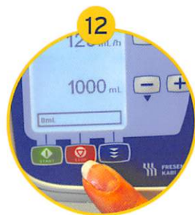
12 To stop feeding at any point, press the stop key. When feeding has finished or your target volume is reached, press the stop key
