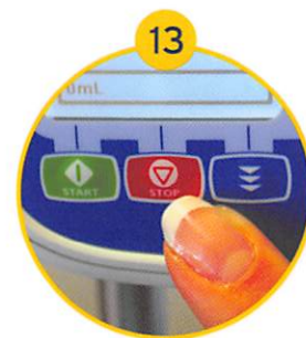
13 If you need to reset the progress bar after target volume is reached, press the stop key for 2-3 seconds
