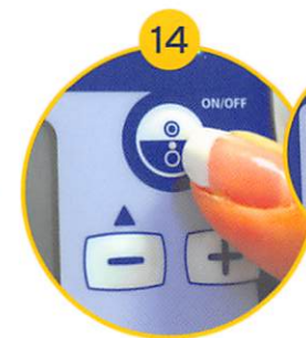
14 To switch off the pump until the countdown is completed, press the on/off button
