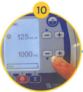
10 Set the target volume by pressing the +/- keys until the desired volume is reached
