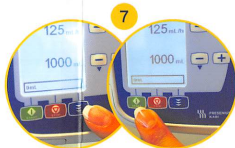
7 Press the automatic priming key, and then press the start button
